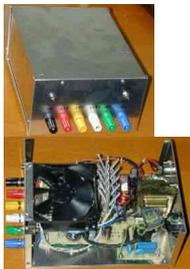
Before I begin, what was I using before? Here are two pictures of my previous station power supply. This consisted of an ex-COMPAQ PC 300W PSU repackaged in an aluminium box with connectors on the front panel.
