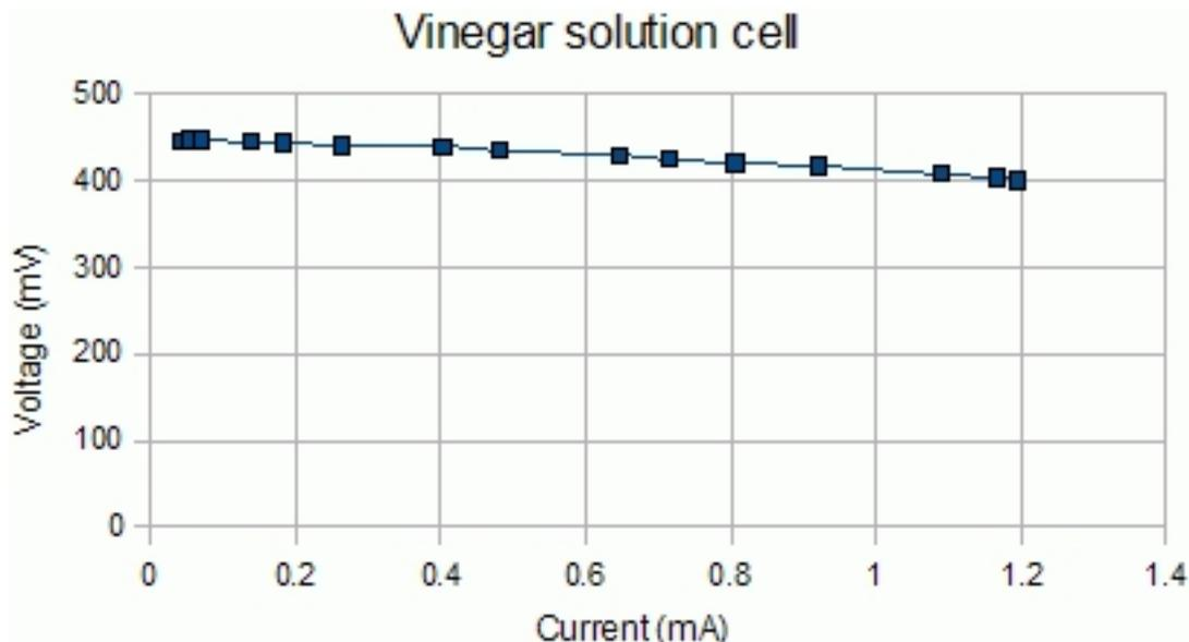
Next comes my vinegar cell. Balsamic vinegar, to be exact, since I had no plain vinegar. I covered the bottom of a new baked bean can with a few mm of balsamic vinegar, put in the orange juice bottle with wire wound around, and filled up with water.
