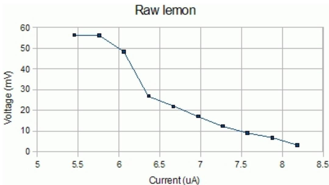
My first attempt at a lemon battery consisted of a standard lemon, fresh from the supermarket, with a copper wire (solid core household cable with the insulation stripped off) poked in one side and a normal steel bolt pushed in the other side. To test this power generation masterpiece, I rigged up a 10k variable resistor in series with a 330-ohm fixed resistor and my two DVM to measure voltages and currents.
