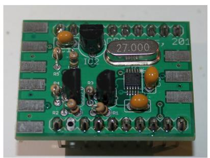
The Si5351A is a relatively recent clock-generator chip manufactured by <u>SiLabs</u>. It can produce three simultaneous independent 50-ohm impedance, squarewave outputs between 8kHz and 160MHz. Configuration of the chip is via a microcontroller with I2C (two-wire) interface.
